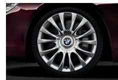
19" light alloy wheels V-spoke 349 l. Front 8.5 J x 19 with 245/40 R 19 tyres; rear 9 J x 19 with 275/35 R 19 tyres.
