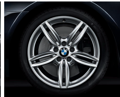
19" M light alloy wheels Double-spoke 351 M with mixed tyres, front 8.5 J x 19 with 245/40 R 19 tyres, rear 275/35 R 19 with 9 J x 19 tyres.
