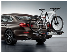
Rear carrier system for transporting up to two bicycles.
