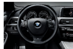
M leather multifunction steering wheel , incl. shift paddles for the eight-speed sport automatic transmission.
