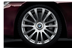
20" light alloy wheels V-spoke 374 l, forged. Front 8.5 J x 20 with 245/35 R 20 tyres; rear 9 J x 20 with 275/30 R 20 tyres.
